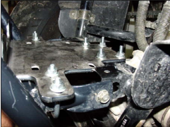
THESE 5/16X1 BOLTS AND 5/16 WASHERS WILL BE SUPPLIED WITH THE WINCH THAT IS PURCHASED.
